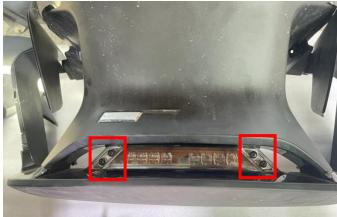
5. Use one end of the matching adapter cable to connect the LED auxiliary light harness plug-in, clip other adapter cables into the trunking on the storage box, fix the storage box on the front bar with the previously removed buckle, and install the grille and other decorative panels.
