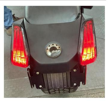
3. Connect the taillight wiring harness with the vehicle wiring harness, and install the license plate bracket back. As shown in figure:
