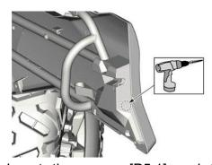
5. Insert the screw [P5.1] and the support washer [P5.3] then pass the screw through the slotted hole.
