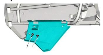
3. Remove and discard the two (2) screws, two (2) nuts and two (2) washers fixing the rear left lower door cover in order to remove it.
