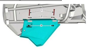
4. Open LH rear door and drill a hole of 30 mm (1-3/16 in) using a step drill where specified below.
