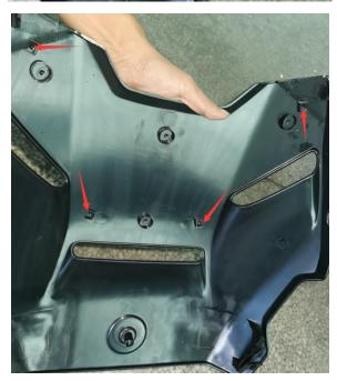
2. Fix the cover decoration plate on the drilled cover with M5\*12 inner hexagon screws, flat pads and square nuts.
