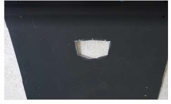
4. Remove the screws from the vent on the aluminum roof and reserve.
