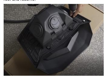
5. And place the plastic bracket into the hole of the aluminum roof. Fix it to the roof with self-tapping screws.
