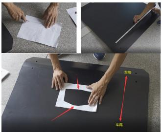
2. Fix the drilling template on the roof with adhesive tape. Open and drill holes by specialized cutting tools and drilling tools.
