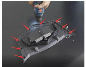
7. After the operation of Step 6, remove the plastic bracket and clean the aluminum roof.
