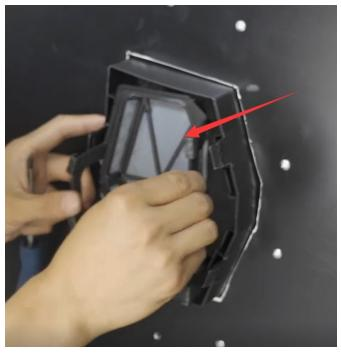
12. Install the rubber baffle on the front position of the vent cover.
