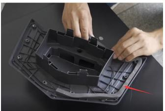
9. Install the bracket with the sealing strip on the roof.
