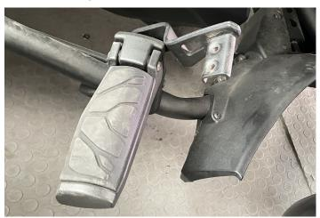
2.Install the new accelerator pedal and fix it with the removed screws, as shown in the picture:
