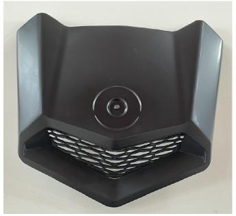
3. Remove the cover of the original vehicle and reinstall the cover with a net. As shown in figure:
