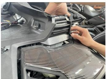
4. Remove the original vehicle fairing, install the fairing with accent light, and then connect one end of the product's adapter to the vehicle wiring harness plug-in and the other end to the fairing wiring harness. When finished, start the vehicle and check if the fairing light is on properly. Finally, the disassembled parts can be installed back to the original position. As shown in figure:
