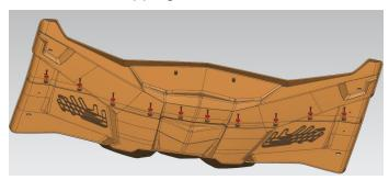
4. Use M5x16 screws, gaskets and nuts to connect the two half roofs in the order shown in the figure.
