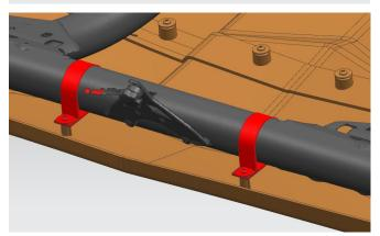
10. Install the clamp on the frame with the screw of M6. The nut is not tightened at first.
