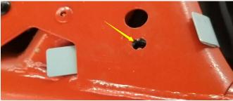
9. Install the clamp at the front of the roof on the frame with a 6mm self tapping screw, and do not tighten the screw first.
