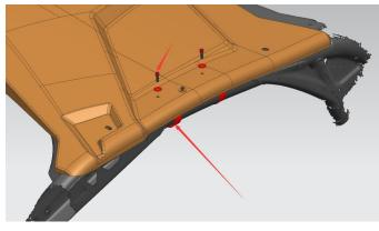
11. The back of the roof is fixed with bake lite handle screw and butterfly nut. After fixing, tighten the screws in step 8, step 9 and step 10.
