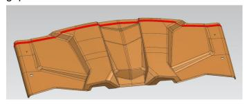
3. Connect the two half roofs with 6mm flat pad and 6x16 self tapping screw.
