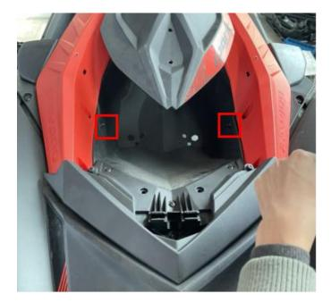
6. There are two bayonets in the middle of the lower frame of the storage box. Press the top of the storage box lid against the bayonet, then
