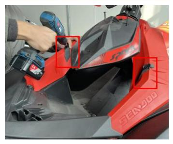
5.Adjust the front and rear orientations of the storage box, and then put it into the motorboat, there are screw fixed points on both sides of the storage box. According to the position of the fixed points, drill holes with a pistol drill (4.5mm drill bit), and then fix it with screws (a flat washer needs to be threaded through the screw), as shown in the picture:
