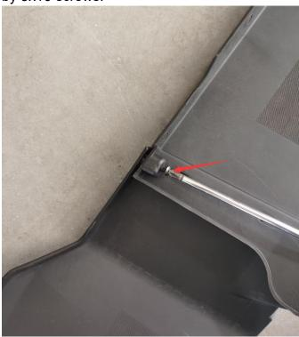
2. Fix the two parts of the fender flare by M6x16 screws as picture.
