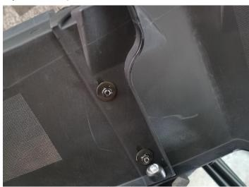
3. Install the fender flare on the vehicle by 5X30 self-tapping screws and flat washers.
