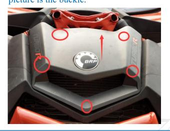
2 Remove the two screws pointed by the red arrows.
