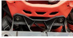
Place the shock tower LED light bar bracket on the water tank bracket and the frame bracket, and install the screws and tighten.
