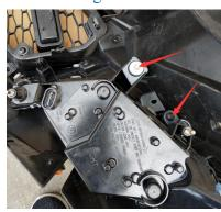
6 Remove the screws pointed by the red arrow and the buckle at the position of the red circle.
