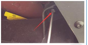
Remove the screw and buckle by the arrow.
