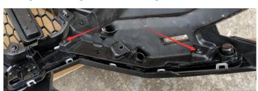
The position light is also connected to the plastic front bumper with 3 buckle. Be carefully, and remove the original lamp.
