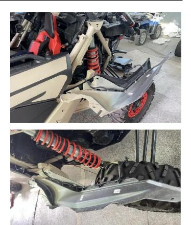
5. Install the new fender deflector onto the trim panel, and then use the vehicle's own screws and accessories to fix it (the other side can be installed in the same way).
