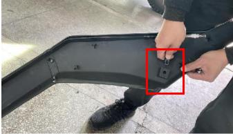
4. Remove the nylon buckle of the rear wheel trim panel, unscrew the screw fixing the vehicle wheel eyebrow, and remove the fender flares.
