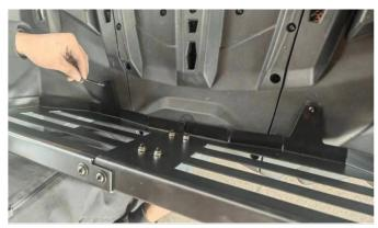
7. Fix the guardrail on the rear carriage with 6 hexagon screws of M6\*30 removed, as shown in the figure, and tighten all the screws.
