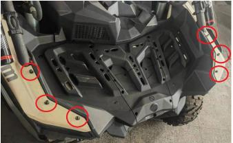
5. As shown in the figure, remove the 2 screws on the original vehicle and the 2 nuts at the bottom for standby.
