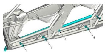
6. Tighten the M10 screws and then the M8 connection screws on the casing.
