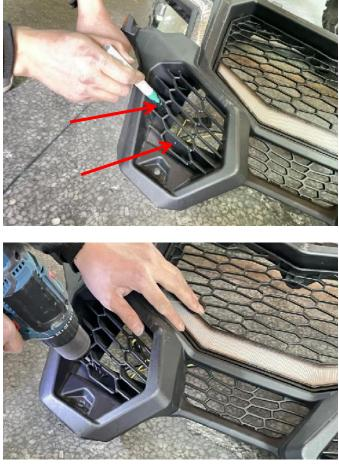
5. Place the mesh grill light, then pass through the fixing hole in Step 4 from the back, fix it with screws, and then use the "L" shaped small bracket in the product accessory package to fix the remaining 2 positioning columns. (The other side of the light can be completed in sequence according to the above steps.)
