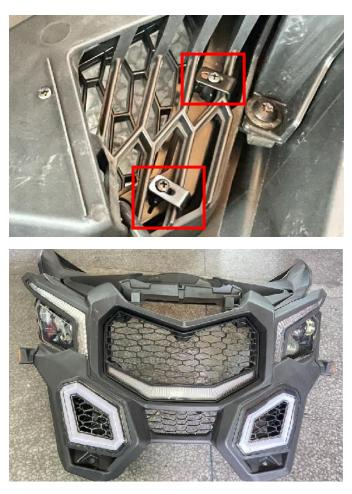
6. Install the installed mesh grill and front fascia back into the vehicle and fix them. Reconnect the harness of the headlight, then connect the harness from the original daytime running light to the matching adapter wire for this light, connect the other end to the vehicle harness, and finally connect the mesh grill light harness.
