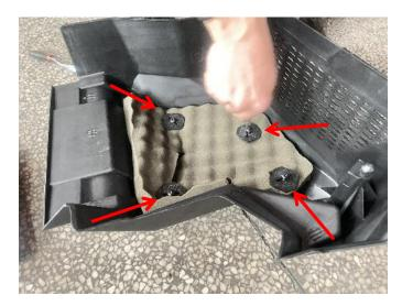
4. Install the new intake hood onto the original vehicle (the fixing clamp on the intake hood needs to be clamped to the front bumper tube).
