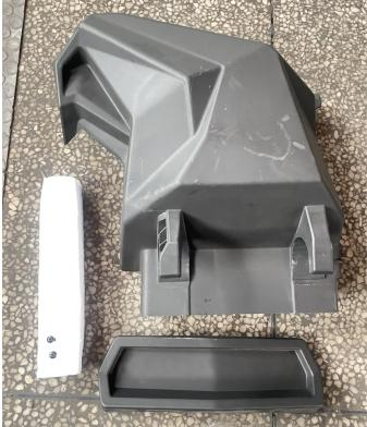
3. First, remove the original air intake mask of the vehicle, take out the built-in filter cotton and place it in the new air intake mask, and fix the filter cotton with the original plastic press plate.
