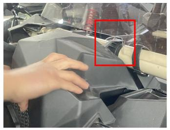
5. Plug the air outlet at the rear seat on the driver's side of the vehicle with pearl cotton from the product accessories, then cover the cover, then use a 3MM drill bit to drill a fixing hole according to the position of the screw hole on the cover, and finally use the screws in the accessory package to fix it.
