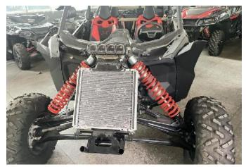
5. Remove the middle net, headlight and daytime running lamp connected with the upper cover plate of the front fascia of the vehicle, then remove the upper cover trim panel of the vehicle, and finally install the new trim panel (The steel clip on the original vehicle trim panel needs to be moved to the new one).
