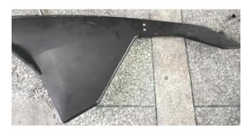
4. Remove the cover plate on the original front fascia and the cover trim panel from the vehicle
