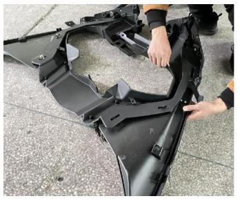
6. After installation, clip the original vehicle's fixing clip back to its original position.
