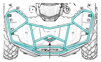
6. After drilling new mounting hole, open front storage box cover to gain access to the underside. Use provided screw w and nut e to secure center rack mount into position.
