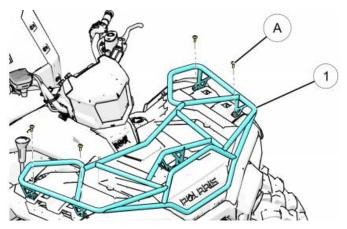
5. Once you have secured the rack you will need to use a drill and 1/4" drill bit to make a new hole for fastening the center support of the rack to the front storage box cover in the location indicated below.
