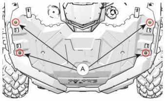
4. Place rack on front storage box cover, align mounting holes and fasten using existing screws A.
