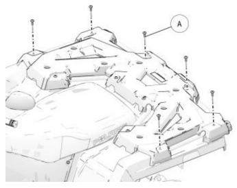
**Note:** Assemble all hardware before tightening rack extender.
