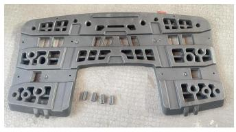
3. Remove the rear rack of the vehicle, and keep the original mounting screws, nuts and iron brackets. As shown below:
