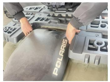
5. Prepare the original medium length screws, insert them into the fixing hole at the end of the rack, put the supporting liner over them and pass them through the fixing hole of the vehicle (both sides of the end need to be fixed in this way), and finally fix them with screws. As
