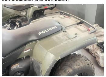
4. Fix the iron bracket (1 long and 2 short) of the original car on the rear rack, and then use the longest original screw to pass through the rear rack, put on the supporting liner, and then install the rack on the car (screws need to be stuck into the original fixing hole on the car),
