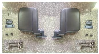
3. Firstly, assemble the supporting mounting bracket of the product on the side mirror (distinguish the left and right sides) and fix it with screws. As shown below:
