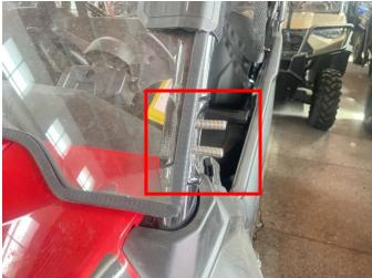
5. Attach the black aluminum bushings of the parts to the screws that just replaced, then install the side mirror on A-pillar and secure it with nuts. (Follow the above steps to install the other side mirror). As shown below:
