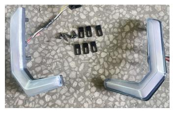
3. First remove the mesh grill of the original vehicle, then install the mesh grill lights, and use the small "L" shaped brackets to fix them. As shown in the picture:
