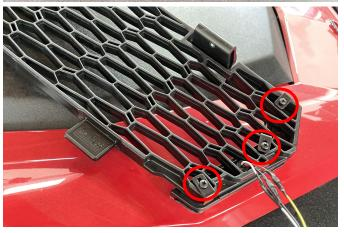
4. Remove the cover of the original vehicle, get the adapter wires out from the package, and connect them with the mesh grill lights separately, and then install the mesh grill on the vehicle, and the extension wire of the adapter wire extends to the terminal post through the gap of the vehicle (the black wire is connected to the negative, and the red wire is connected to the daytime running), and finally install the cover. As shown in the picture:
