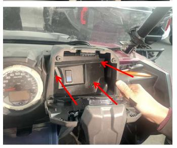
2. Use nylon expansion screws to fix the holes. As shown below:
