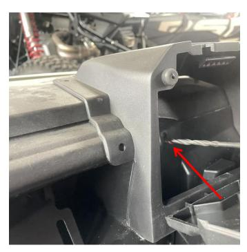
2. Use nylon expansion screws to fix the holes. As shown below:
