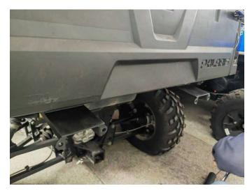
4. Fix the mounting bracket 6 at the bottom of the frame with four M6\*25 flange self-tapping screws. Install the bar body on the iron support with four M8\*65 hex socket screws and four M8 locknuts, and tighten all screws.
