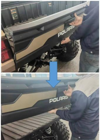
2. Install part 6 on the lower bracket of the rear of vehicle with two M8\*90 screws and two M8
