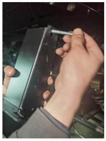
3. Fix the mounting bracket 6 at the bottom of the frame with four M6\*20 self-tapping external hexagon screws. Install the bar body on the iron support with four M8\*65 hex socket screws and four M8 locknuts, and tighten all screws.
