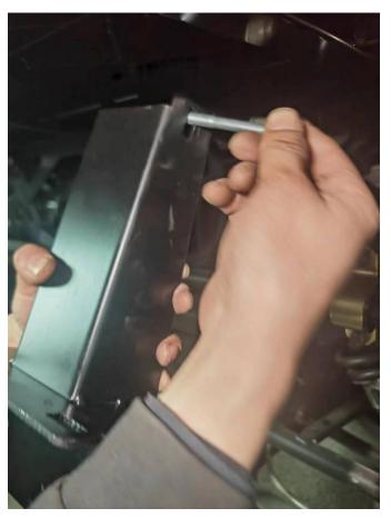
2. Fix the mounting bracket 6 at the bottom of the frame with four M6\*20 flange self-tapping screws. Install the bar body on the iron support with four M8\*65 hex socket screws and four M8 locknuts, and tighten all screws.
