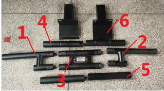
2. Assemble Part 1, Part 2 and part 3 by connecting casing 4 and connecting casing 5 with eight M8\*55 hex socket screws and eight M8 locknuts. The direction of casing is shown below:
