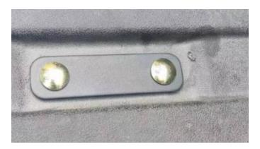
4. Install the rear bumper with 4 M8 jam nuts and M8 carriage screws, and tighten all screws. As shown below:
