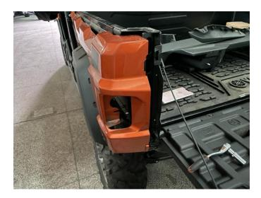
3. Install the new taillight on the car, fix it with the nut flat pad of the original car, and then butt the taillight wiring harness again with the vehicle wiring harness. At this time, you can start the car, check whether the taillight function is normal, and install the decorative plate back to the original position after completion. (Replace the taillight on the other side by following the same steps as above.) As shown below:
