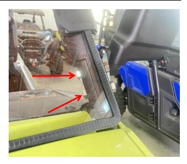
4. Finally, adjust the angle of the side mirror, and then tighten the nut in step 2. (The side mirror on the other side can be installed according to the same steps above). As shown below:
