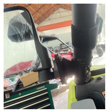
5. Clip the matching mounting bracket of the interior mirror onto the front bar of the original vehicle roof, then pass the fixing screw on the back of the interior mirror through the fixing hole on the mounting bracket, and finally fix it with a nut. As shown below:
