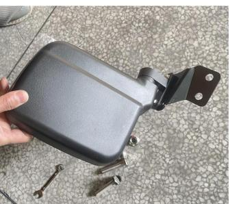
3. Unscrew the screws on the guard bar of pillar A of the original car, use the trombone screws matching the side mirror, pass through the support hole of the side mirror, put on the liner and install on the guard bar of pillar A, and then tighten the nuts. As shown below:
