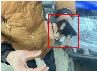
4. Finally, adjust the angle of the side mirror, and then tighten the nut in step 2. (The side mirror on the other side can be installed according to the same steps above). As shown below:
