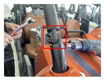
3. Assemble the corresponding side mirror on the mounting bracket and fix it with matching screws.(The side mirror on the other side can be installed according to the same steps above)As shown below:
