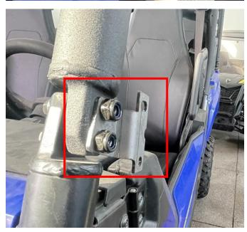
3. Assemble the corresponding side mirror on the mounting bracket and fix it with matching screws.(The side mirror on the other side can be installed according to the same steps above)As shown below:
