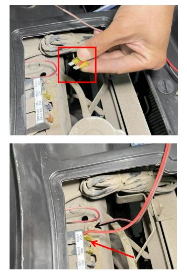
5. Connect the conversion cables of the power supply, then pull it along the gap of the vehicle to the front bumper panel, and connect it with the lamp wiring harness on the panel successively (connect the same color wiring harness), and then install the new panel on the vehicle, Finally cover the electrical box and storage box lid. As shown below:
