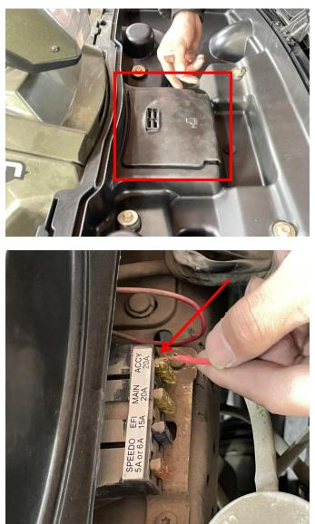
4. Prepare the conversion cables for the product. Peel off the top of the red and black wires. Stick the copper wire of the red one on the fuse, and then insert the fuse back to the original position. Wrap the copper wire of the
