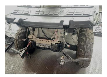
4. Remove the headlamp from the front fascia of the vehicle and install it on the new front fascia in the original way, as shown in the figure:
