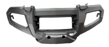
**3.** First remove the cover plate of the front fascia of the vehicle (from the bottom right corner of the cover plate from inside to outside), then unscrew the screws fixing the front fascia, and remove the front fascia (disconnect the wiring harness plug-in of the headlamp of the vehicle before removing the front fascia). As shown below:
