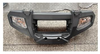
5. Reassemble the front fascia of the installed headlamp to the vehicle, connect the wiring harness plug-in of the headlamp, and finally install the front fascia cover plate. As shown below:
