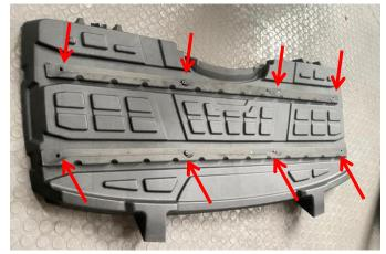
5. Install the storage cover with the iron bracket back on the vehicle. You can fix the upper cover with the original connecting pin of the vehicle, or with the screws of the product, and finally assemble the front fascia of the
