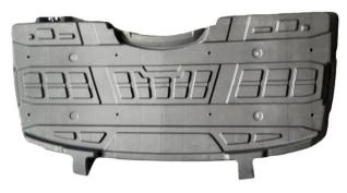
3. First remove the front fascia of the vehicle (Remove the upper cover of the front fascia from the bottom right corner of the cover plate from inside to outside. Disconnect the wiring harness plug-in of the headlamp before removing the front fascia.), then open the upper cover of the storage box, and remove the storage cover after prying out the connecting pin on the hinge bracket with a tool. As shown below:
