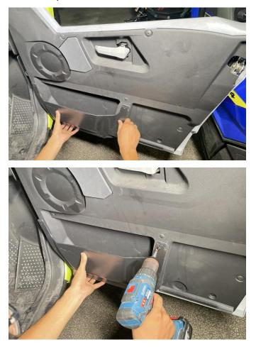
2. Drill a screw hole by a 3MM drill bit as indicated in the picture, and then tighten the screw. (The storage box on the other side can be installed as the same steps 1-2) As shown in the picture:
