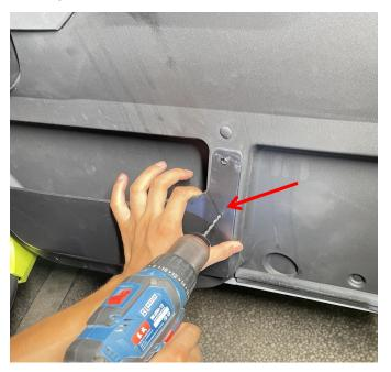
3. Distinguish the left and right sides of the product, and then place the storage box at the installation position of the rear door panel. Fix it with the screws provided with the product. (Follow the same steps to install the storage box on the other side). As shown in the picture:
