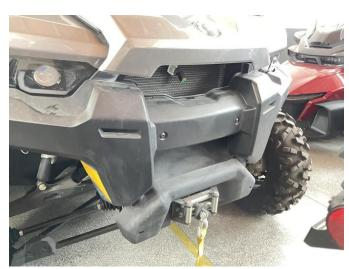
3. Install the grille light onto the grille and secure it with an "L" shaped bracket from the back. As shown below:
