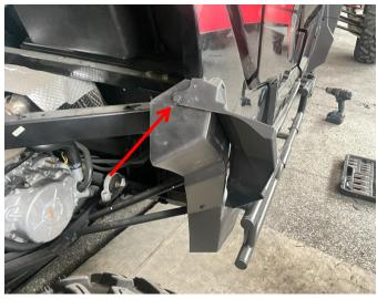
2. Follow step 2 of front fender flares, use a 6mm drill bit to drill the remaining positioning
