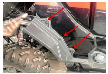
3. Assemble the rear fender flares of the separate parts into a whole with screws. As shown below:
