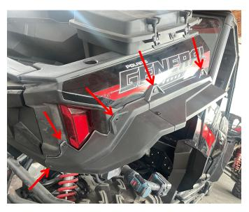
5. Finally, fix the hole at the head of the fender flare with self-tapping screw (the other side of the fender flares can be installed in the same way as steps 1-5 above). As shown below:
