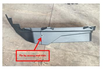
4. Place the assembled fender flares on the stock fender flares of original vehicle, drill the fixing holes according to the positioning holes on the fender flares with a 6mm drill bit, and then fix them with snap fasteners. (Drill the fixing hole in the middle first, and fix it with snap fastener first, which can effectively prevent the fender flares from moving when drilling other holes). The other side of the fender flares can be installed in the same way as above. Figure as below:
