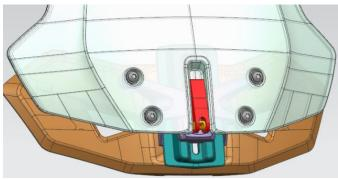
5. The whole device can be tightened by tightening the screw behind the trigger.
