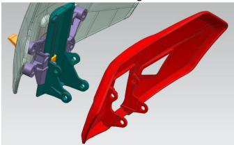
3. Fix the windshield on the frame with screws as shown in the figure.
