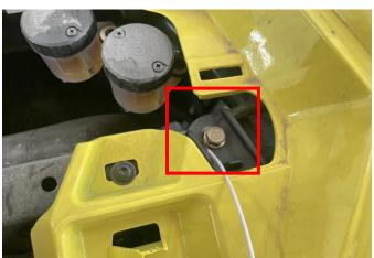
3. Prepare another extension cable, insert the extension cable through the reserved hole at the cover into the cockpit, and then pull the extension cable through the lower part of the instrument panel along the gap to the ACC electrical box under the steering wheel (it can be crossed through the gap at the connection between the steering wheel and the operating lever).
