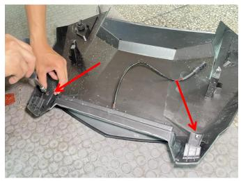
3. Install the cover of the spotlight back to the original vehicle. When installing the spotlight, firstly, thread the spotlight harness through the gap beside the kettle to the front center net, connect it with the broken skin of the wire harness of the mesh grill light, and do insulation protection. Finally, start the vehicle to check whether the spotlight is turned on normally. After checking, install back the mesh grill of original vehicle and fix the cover. As shown below:
