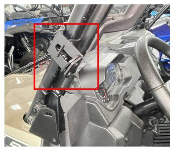
3. After adjusting the side mirror to an appropriate Angle (there is a screw at the bottom plug of the side mirror, you can loosen the screw to adjust the Angle of the side mirror), install the mirror on the mounting bracket, and fix it with screws. Install the side mirror on the other side as above steps. As shown below:
