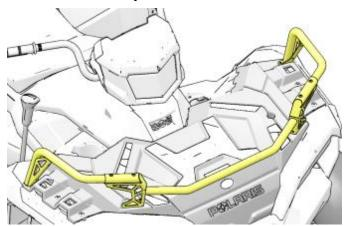
9. Reinstall two screws (B) removed in (Step 4) on front rack (A) through the rack extender assembly as shown.
