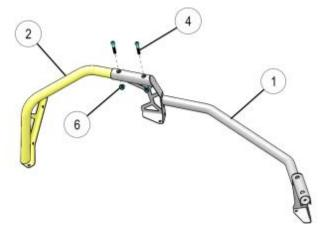
3. Repeat (Step 2) for RH rack extender ③ installation.
