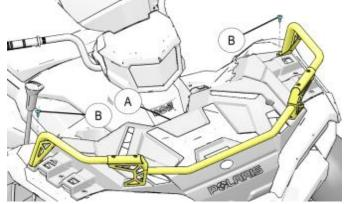
10. Tighten all fasteners. Secure front rack using rubber latches (C). The installation is complete.
