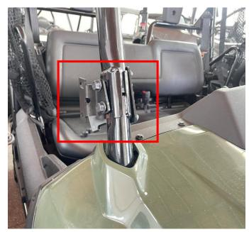
4. Fix the side mirror on the mounting bracket using the matching screws and nuts (the screws must be covered with flat pads. Then adjust the proper angle of the mirror, and tighten the nuts. (The other side mirror is installed in the same way as above). As shown in the figure.
