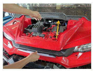
4. After finding the wiring harness plug-in reserved by the vehicle, connect it with a wiring harness plug-in on the grill light. Then fix the other wiring harness on the grill light on the negative plate of the battery by using the screws and nuts in the accessory bag. After the completion, first test whether the light is on normally, and after confirming that it is correct, the grill light can be embedded in the grille of
