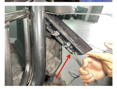
8. Prepare the other adapter wire #2 in the product accessories, connect the extension wire after breaking the skin (connect with the same color), and make insulation protection.
