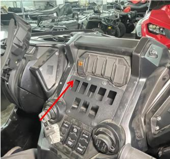
6. The newly connected extension cable is also threaded into the co-pilot through the gap at the front cover, and then pulled along the gap to the outlet hole at the rear seat, and to the rear taillight from the outlet hole. As shown below:
