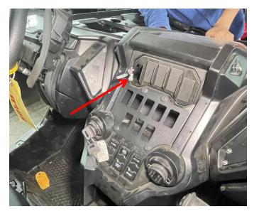
5. The wiring harness through the cab will be inserted on the wiring sheet of the control switch in the order, as shown in the picture. Then the control switch will be placed on the switch panel. (If the switch hole is small, use a utility knife to make the hole larger). As shown below:
