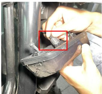
9. Find the wiring harness plug-in reserved by the vehicle at the front cover, disconnect the plug-in at the female end, and then connect the corresponding plug-in on the conversion wire #1 to it. Finally, reinstall the decorative plate and front cover. As shown below:
