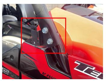
3. Fix the side mirror on the mounting bracket using the M6\*20 screws and matching flat washer nuts in the accessory package. (The side mirror on the other side can be installed in the same way.). As shown below:
