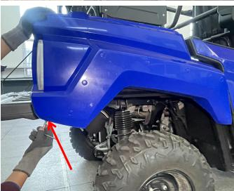
3. After disconnecting the wiring harness plug of the original tail light, remove the decorative panel, unscrew the fixing screws of the original tail light, remove the original tail light, and then replace and install the new tail light on the decorative panel, and then use the original vehicle screws for fixation. As shown below:
